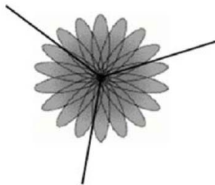
Fig. 1. Coverage pattern of switched beam antenna system.
