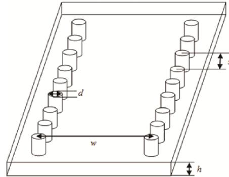
Fig. 2. Substrate Integrated Waveguide
