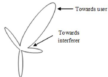
Fig. 1. Beam formation for adaptive array antenna system.
