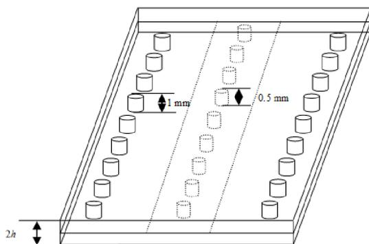
Fig. 3. Structure of Substrate Integrated Folded Waveguide.
