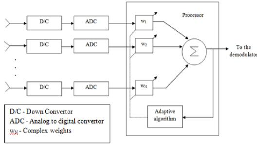
Fig. 2. Basic block diagram of adaptive array system.
