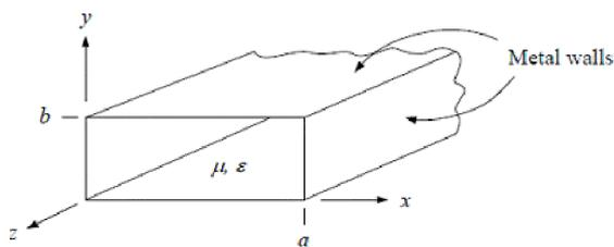
Fig. 1. Non planar classical rectangular waveguide.
