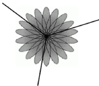
Fig. 1. Coverage pattern of switched beam antenna system.
