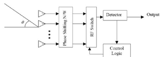
Fig. 2. Basic block diagram of a typical switched beam system.
