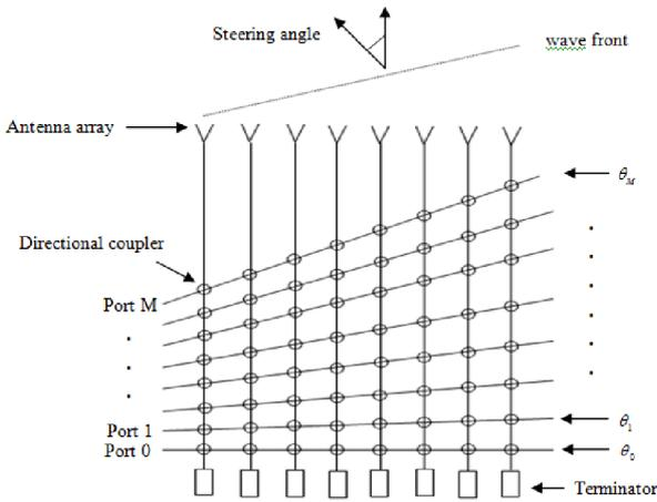
Beam forming network implemented by Blass matrix array.
