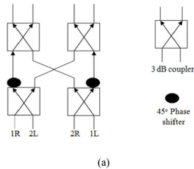
Fig. 1 (a) Schematic of  $4 \times 4$  Butler matrix array.
